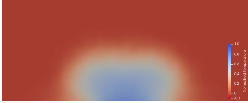
Fig. 6 Normalized temperature \theta in the flat plate region at x/D = 5 for the baseline 30^\circ LES.
